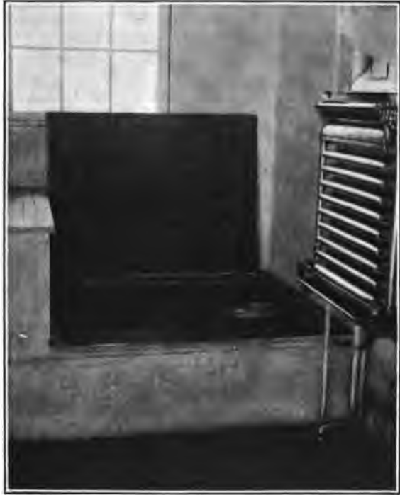
FIG. 6.—Homemade cement tank for cooling milk and cream.
